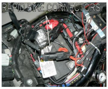
3. Connect the Rapid Bike wiring in-line with the stock connectors.
