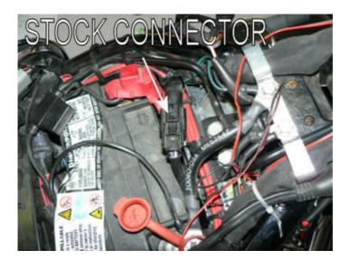
2. Locate the connectors of the lambda sensors.
